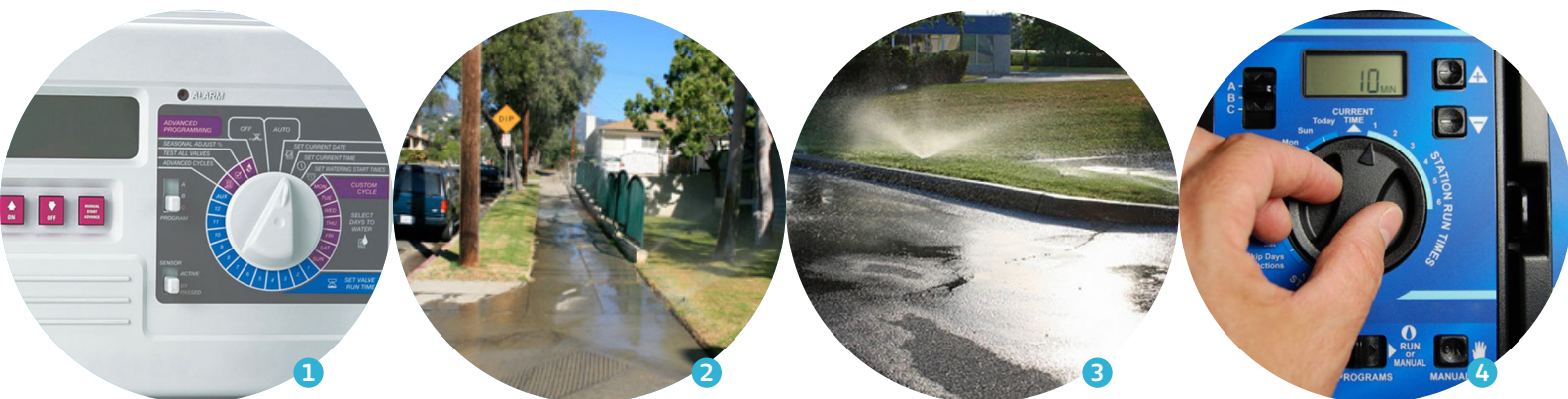
1. Irrigation controller 2. Overspray 3. Overspray 4. Programming your irrigation controller
