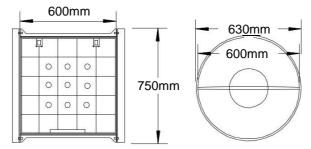
In ground access lid. Cast iron concrete Infill as per AS3906 Above ground access lid. Screw type, polypropylene.
