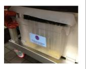
Slide clean canister into cavity, lift & lower to lock canister lip into place. Canister MUST be pushed fully down allowing the rubber blade good contact with the grease roller.
