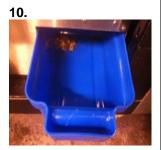
Slide catchment draw out, located on the RHS of Grease Shield unit
