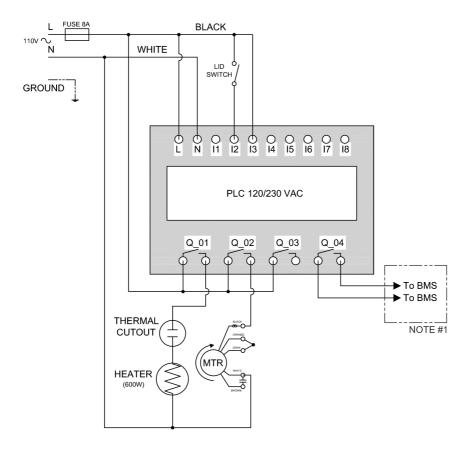
NOTE #1: OPTIONAL - If connecting Output 4 (normally closed contact) to the BMS (Building Management System) ensure that the maximum breaking voltage (5-30VDC, 24-250VAC) and maximum breaking current (8A) are not exceeded
