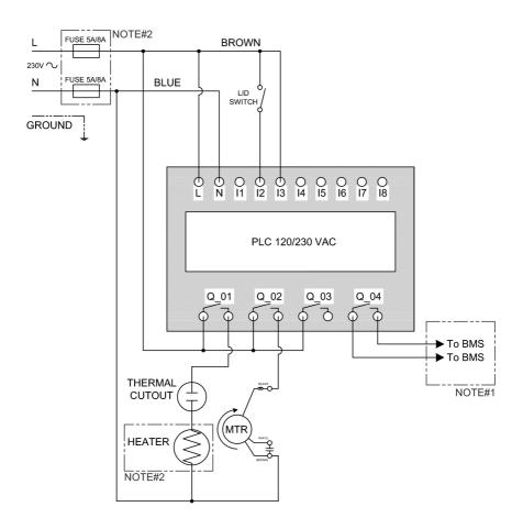
**NOTE #1**: OPTIONAL - If connecting Output 4 (normally closed contact) to the BMS (Building Management System) ensure that the maximum breaking voltage (5-30VDC, 24-250VAC) and maximum breaking current (8A) are not exceeded
