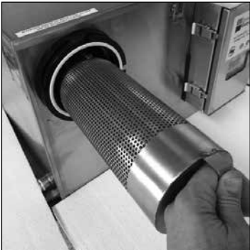
Next remove the strainer by simply sliding it forward.
