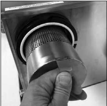
Shake off excess water before removing strainer by turning it while still in its internal cage mount.
