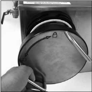
To unlock the cap rotate it counter clockwise using the hand grips.
